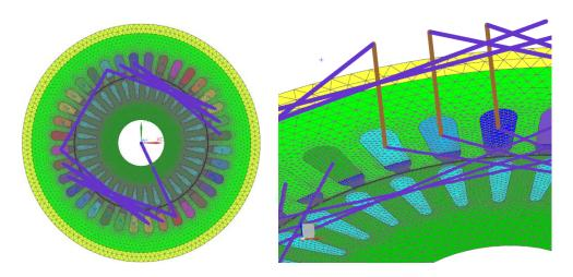
Picture: Automatically generated FEM Model: Meshes and Circuits for the Windings
